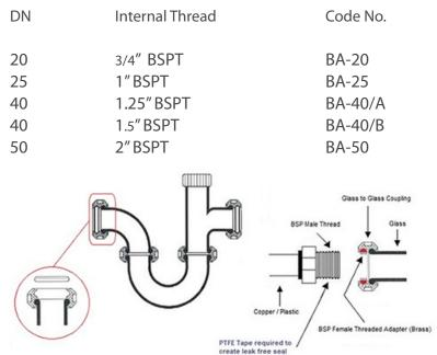
The easiest and most economical way of connecting to other materials is by utillising the standard BSP thread. As the majority of AHU manufacturers now fit BSP male threads to the drain pans as standard on their units, SGL have moved to make this its preferred method of connection: A simple 'O' ring - "BSP threaded adapter" is inserted into a standard glass/glass coupling, replicating the profile of the glass.
