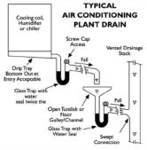
Inspection of the traps e.g. seal depths can be easily monitored due to the transparency of glass, dosing points allow for filling / cleaning. The self-cleaning nature of these traps helps prevent colonisation of sediments such as rust, scale, sludge and algae from providing the nutrients that support the proliferation of legionella.
